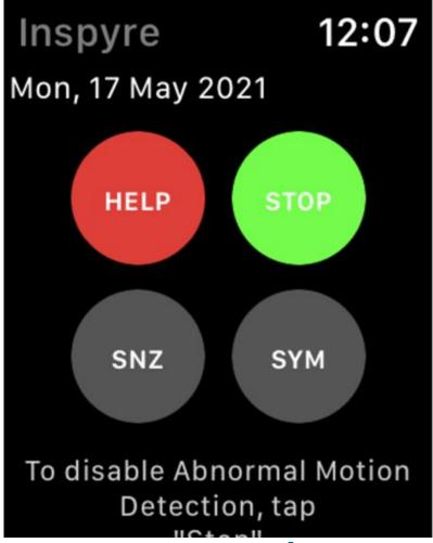
When the Inspyre app on the watch detects abnormal movements, it vibrates on the user's wrist and a cancel button appears. Audible alarms, text, and phone call alerts are automatically sent to the contacts that the user has chosen.
